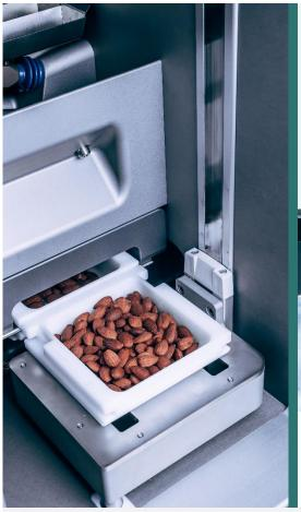
After each tray has been filled individually, it spreads its load over the buffer chutes on the first level of the oscillating dosing system, a brand-new technology developed and patented by Mecaniek Chevalier.
