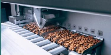
The buffer chutes supply the dosing chutes underneath. The dosing chutes deposit the carefully measured amount of granular products per channel. The product is then released with meticulous precision: in the perfect spot, at the right moment. Each channel of the oscillating dosing system works entirely independently in a closed loop with individual sensors.
